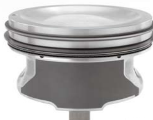
Sumped 9.1:1 Piston Cast hypereutectic coated skirt piston with sump in dome for compression control.
