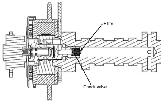
Oil flows through #2 cam bearing, into center of camshaft, through check valve and filter in valve, through oil control spool valve which directs oil into the correct phaser cavity: either advance, retard, or both (hold position).
