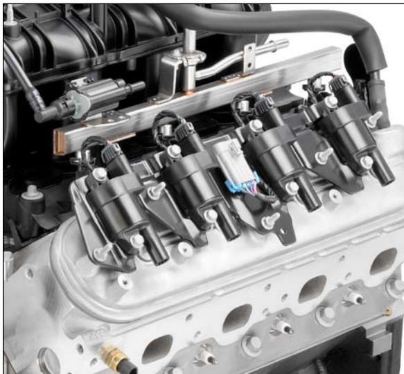
An advanced coil-near-plug ignition system ensures a powerful spark is precisely delivered to each cylinder.
